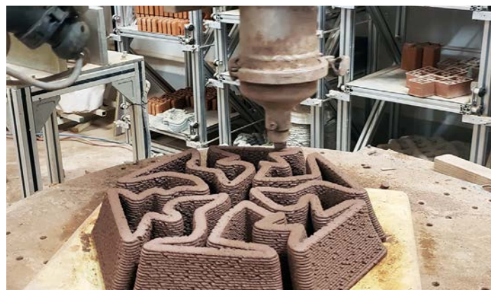
Robotic 3D clay printing method. Source: Chen Zhaowei; Centre for Chinese Architecture and Urbanism; Fabrication and Material Technologies Lab.
